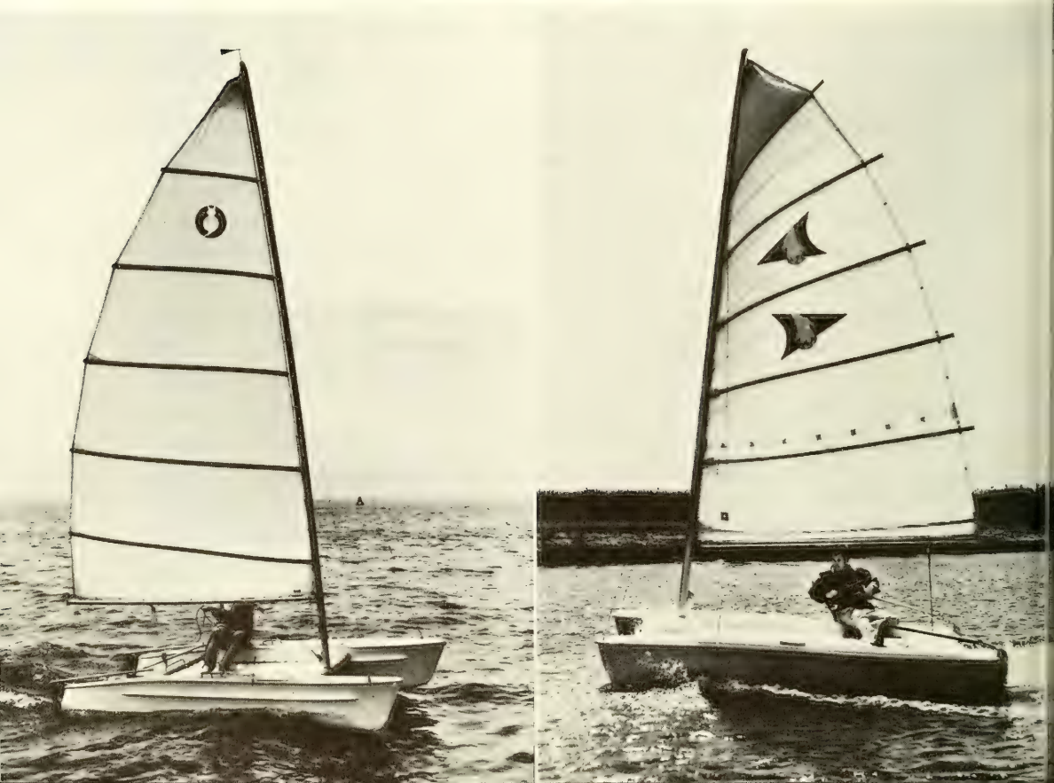
Two one-design catboat rig catamarans: the Aero Cat (left) and the Whisker (right)
